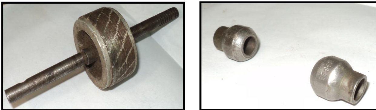
Fig. 3 Domestic Table Fan Rotor and Journal Bearings
